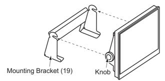
Adjust the angle of the monitor unit and fix the knobs tightly.
